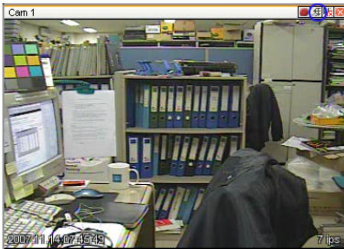
Among the icon on top of video on monitoring, click 'PTZ' to activate interfacing to control Pan, Tilt, Zoom, and Focus. But, when PTZ camera is connected and ready to set PTZ, the button is activated to use the functions.
