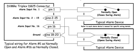
**Normally Open and Normally Closed Connections**
