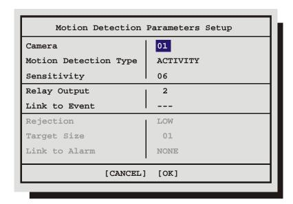
Navigate in this menu using the **Jog** to select the field and the **Shuttle** to change the parameters.
