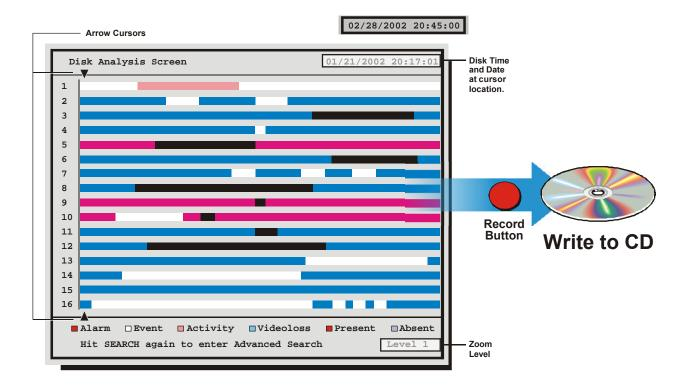
Rotating the **Jog** moves the two arrow cursors across the representation of the recorded video. As the cursors move across the screen the corresponding disk time is indicated in the upper right of the screen. The video representations are color-coded by category. Rotating the **Shuttle** expands (Zooms) the display. The Lowest level (most detail) is indicated on screen with an **(L)**. Pressing the **Enter** button will start Playback from the cursor location.
