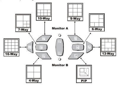
The multiscreen display is limited to the number of camera inputs on the unit.
