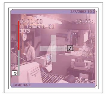
This screen overlays the current playback video and allows the user to enable or disable motion detection on the screen within blocks that form a 16 x 16 grid.
