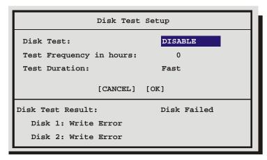
Use the **Jog** to move between the menu fields and the **Shuttle** for the selections within the fields. When satisfied with the selections select **OK** and press the **Enter** button to execute.
