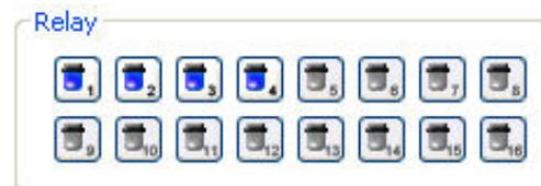
It can On or Off Relay of the unit. Click the number button to activate Relay On, then the icon changes from Blue to Orange color.
